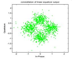
Fig.10.constellation diagram of the outputs with the linear equalizer
