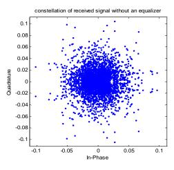
Fig.9.constellation of received signal without an equalizer
