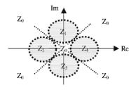
Fig. 7. Boundary of the equalizer output constellation.
