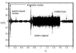
Fig.2.Received signal with noise and reflection
