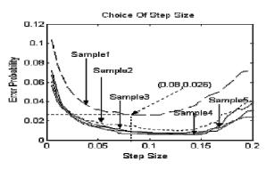
Fig.8.error probability with different step size
